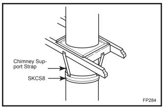
Fig. 9 Chimney support installation
